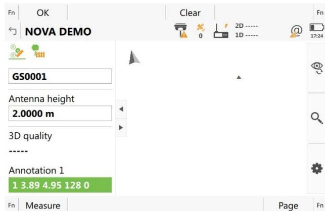
Measurement of points can be done manually but it may be more efficient to measure points every few seconds or over a defined distance. To do this requires auto point measurement to be defined.
