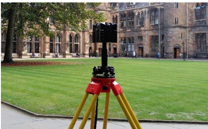
Img. 02.01 and Img. 02.02 LaserScanner and iSTAR station.
