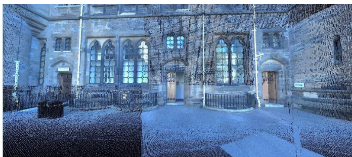
Img. 05.02. Visualisation of Coloured Point clouds with laser scanner internal camera data in TruView from Leica Cyclone 9.1.
