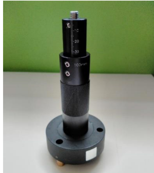
Img. 02.03. Adaptor rod and Tribach setting to achieve the right position for works with Leica P40 laser scanner.
