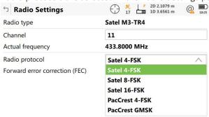
There are many factors which play a role in transmitting and receiving data between digital radios. (e.g. Height of base radio antenna above the surface, Forward Error Correction (FEC), Output power (Tx)...and much more)
