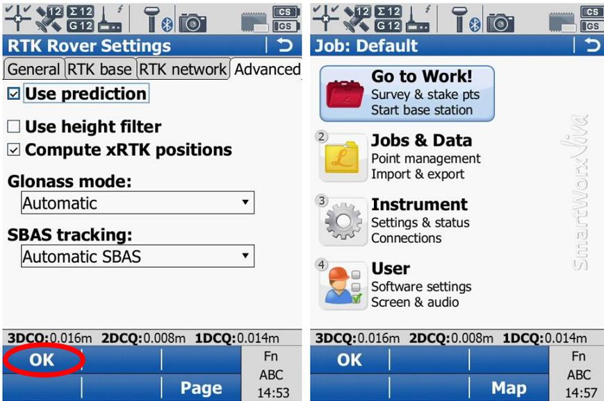
RTK Data link should now be initialized. To verify the RTK settings, check the position icon at the upper left corner. From the main menu, press the Star key, then RTK DATA LINK STATUS to verify the RTK corrections are being received.
