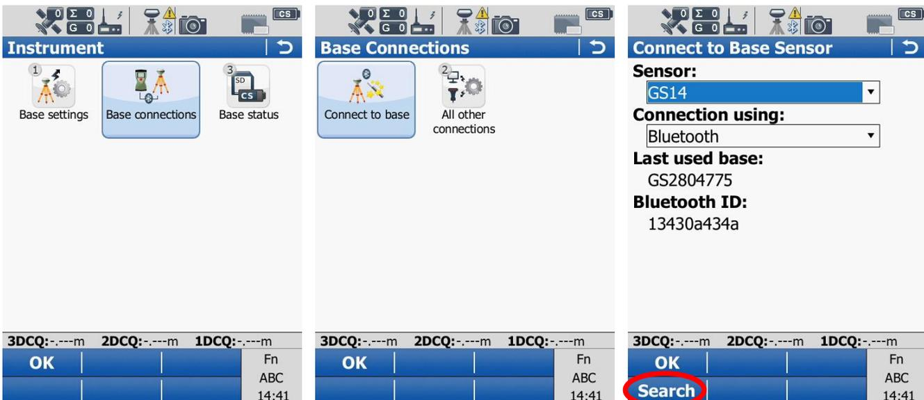
The controller should find your new base. **NAME: GS2804775**. Highlight it and tap **OK**. The controller should now connect to the Base and return you to the Base Menu. Tap **Instrument**, then **Base Connections**, then **ALL OTHER CONNECTIONS** to set RTK Base Connection Settings.
