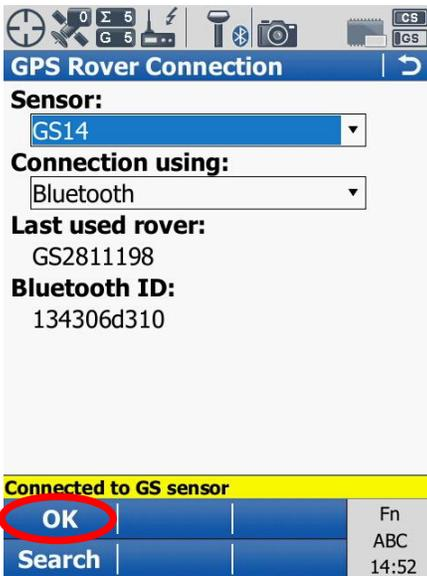
Now, we need the Rover to receive the RTK corrections from the Base. From the Connection Settings menu, tap **GS CONNECTIONS** and highlight **RTK ROVER**. Tap **CNTRL** to set the channel. *Remember, the channel must match the Base channel.* Tap **OK** to return to Connection Settings. Tap **EDIT** to enter the RTK Rover settings.
