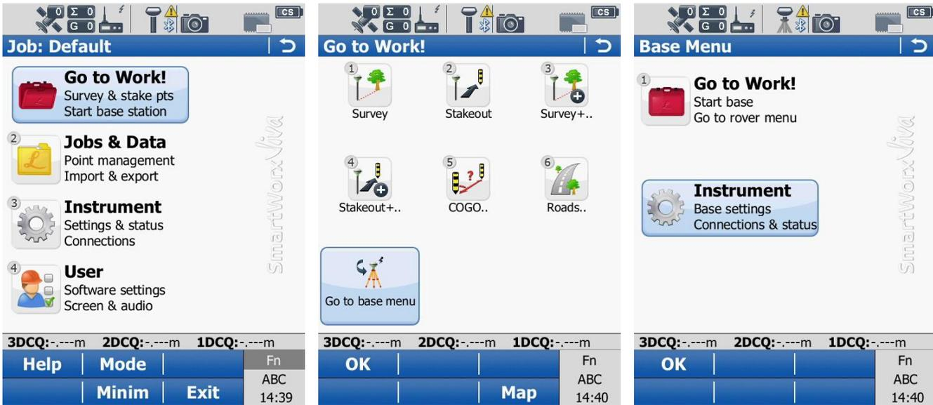
From the Base Menu, select INSTRUMENT, then BASE CONNECTIONS, and then CONNECT TO BASE. In the Connect to Base Sensor menu you should see the ID of your other base. To find the new base tap SEARCH.
